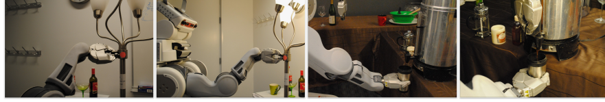
Fig. 7: Examples of transferred trajectories being executed on PR2. On the left, PR2 is able to rotate the 'knob' to turn the lamp on. On the right, using two transferred trajectories, PR2 is able to hold the cup below the 'nozzle' and press the 'lever' of 'coffee dispenser'.
